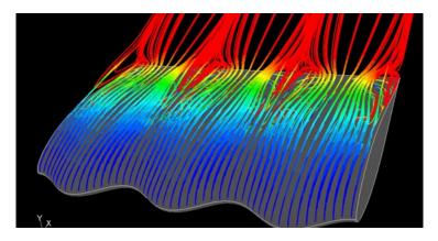
Figure 5: Streamlines displaying tubercle high velocity channels<sup>G</sup>
